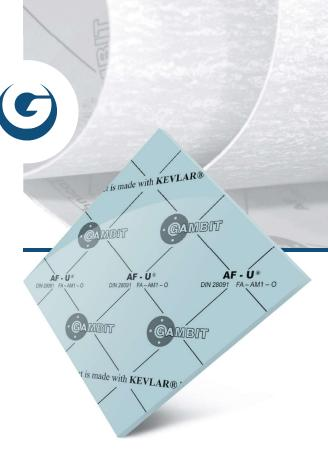
A sheet designed for sealing in medium temperature and medium pressure applications. Water, steam, kerosene, fuel, and oil resistant, among other media.
