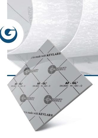
Specially selected components and structure of AF-GL® gasket sheet ensure high tightness of a joint and resistance to a whole range of media, including steam, water, fuels, oils, solutions of salt as well as weak solutions of acids and bases. Thanks to application of a unique composition of fibres and fillers, gaskets made of this material feature higher resistance to operation in steam.
